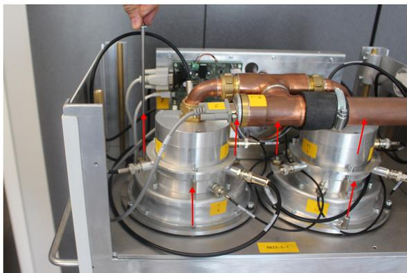
5. Disconnect the **DB9 power and USB communication cables** from the TOP DAQ and pull the cables through the hole in the charger filter unit base plate.
