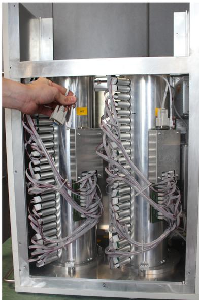
12. Lift the **outer shell of the analyzer** and place it upright on a table. The central electrode remains in place.
