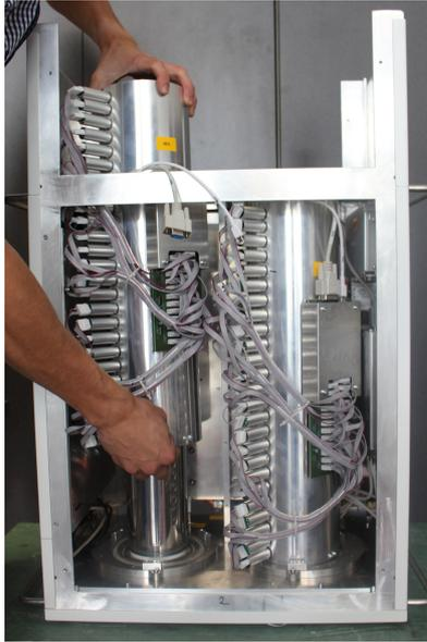
13. Clean the **central electrodes** inside the instrument and **collecting electrodes** in outer shell that was lifted away. Use soft tissue paper or cloth and alcohol. Prefer materials that do not leave fibers.
